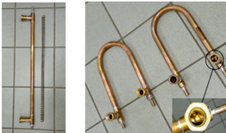
Figure 3: Pictures of the manufactured double pipe straight and U-bend heat exchangers with helicoidal turbulator.
