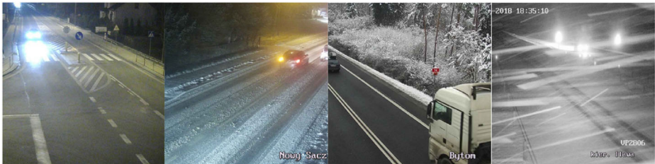
Fig. 13 Correctly classified images. From left to right: dry, snow, wet, snow
