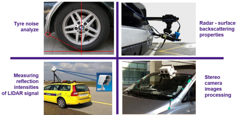
Fig. 4 Photos of experimental setups for determining road surface condition
