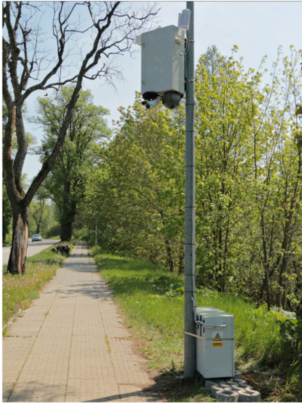
Fig. 3 Photo of the measuring station of the intelligent road sign with CCTV camera sensor attached to the bottom of its housing
