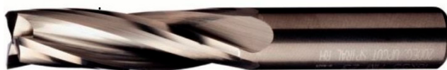
Figure 5. Mill cutter used for wood milling process at the SCM Tech Z5 milling centre.
