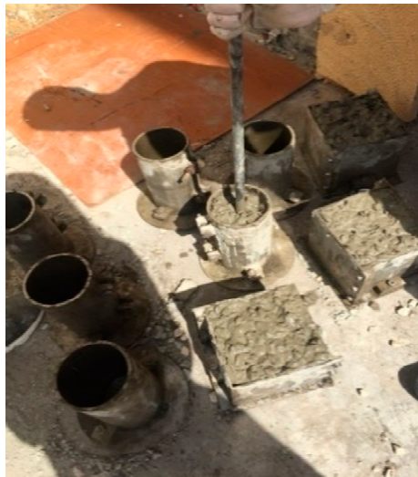
Figure 3. Casting and compacting.
