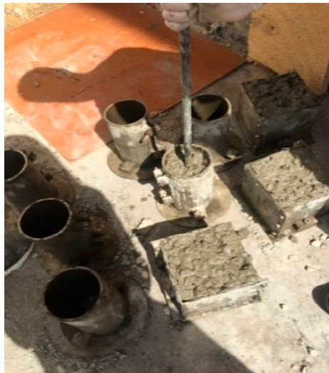
Figure 3. Casting and compacting.
