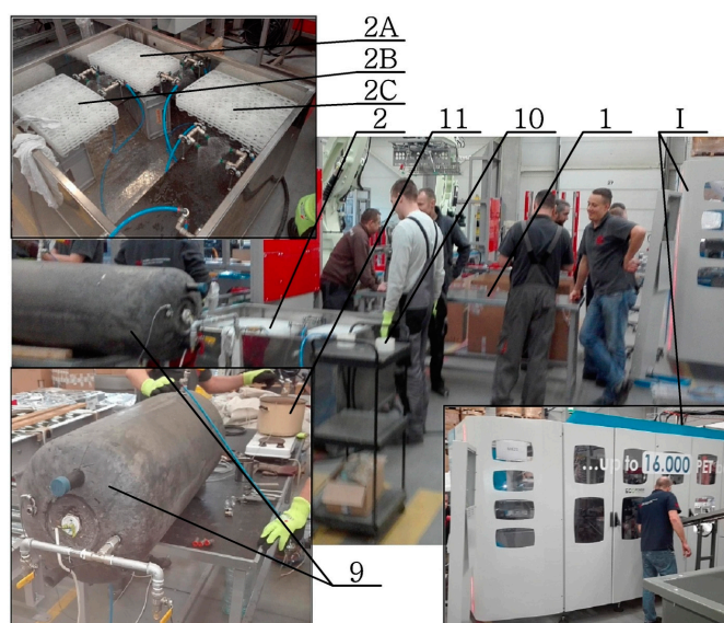
Figure 2. Measuring station for filling, annealing, and cooling of manufactured bottles (the numbering shown in the figure refers to the numbering shown in Figure 1 and Table 1).
