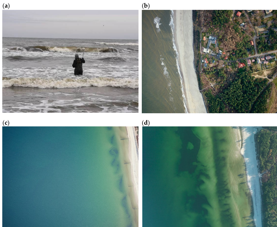
Figure 3. Representation of Red–Green–Blue (RGB) images specifying the bathymetric scanning conditions on a five-point scale: (a) 1–2, cloud cover and large waves make topographic–bathymetric
