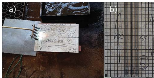
Fig. 2. Test plate during straightening process (a) and surface after process (b)
