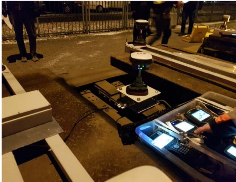
11. GNSS receivers mounted on racks
