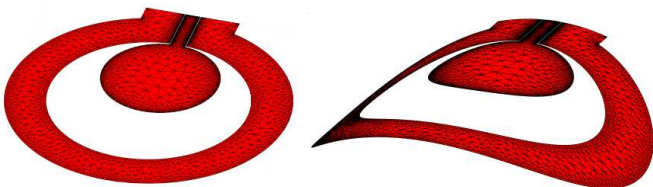
Fig. 1. Mesh of planar antenna and the same mesh after projection onto conformal surface
