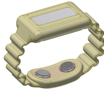
FIGURE 5. The wristband model containing electronic components and electrodes.
