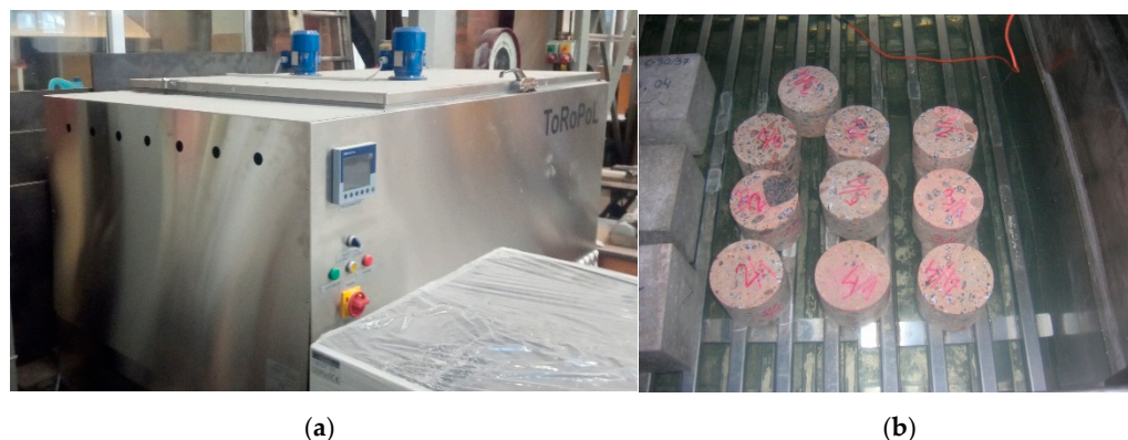
Figure 4. Frost resistance tests: (a) view of freezing chamber; (b) view of concrete specimens inside the freezing chamber.
