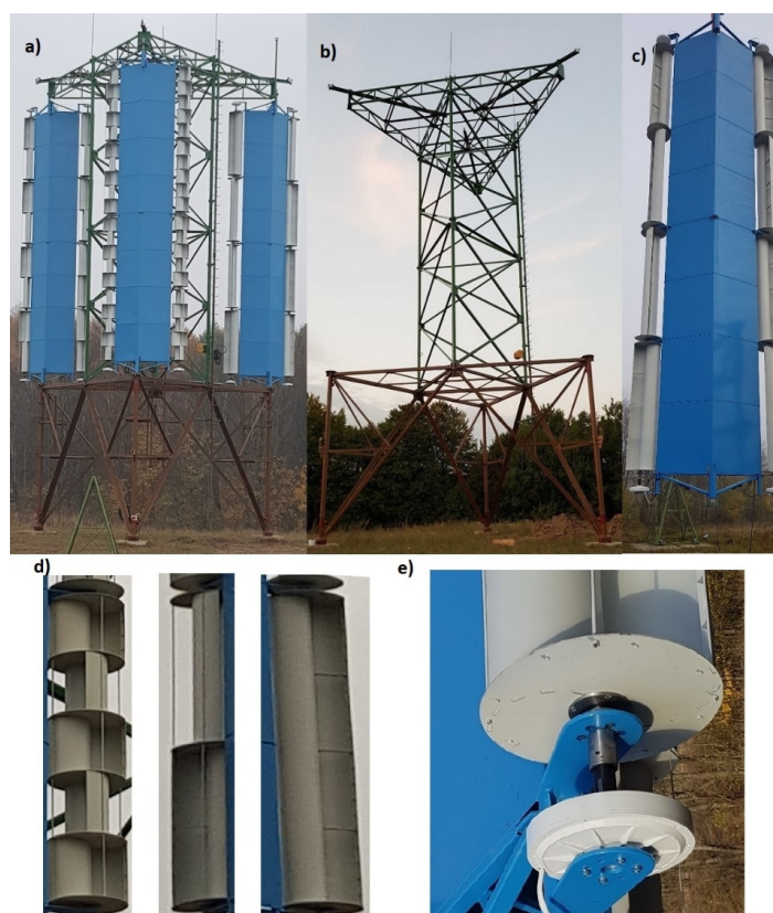
Figure 2. (a) Wind turbine; (b) wind turbine tower; (c) wind turbine structure; (d) rotors 1-, 2-, 5-modules; (e) generator.
