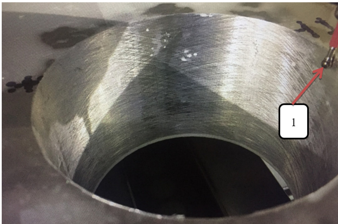
Figure 14. Example of a honed surface without texture defects, 1—probe tip.
