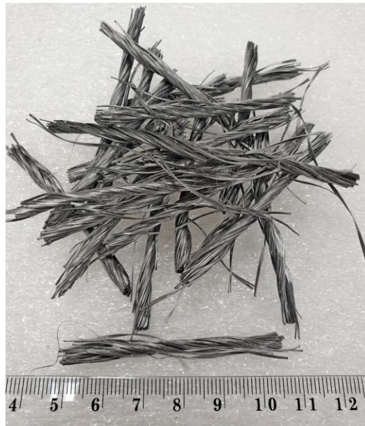
Figure 2. Photograph of twisted-bundle macro-polyolefin fibres
