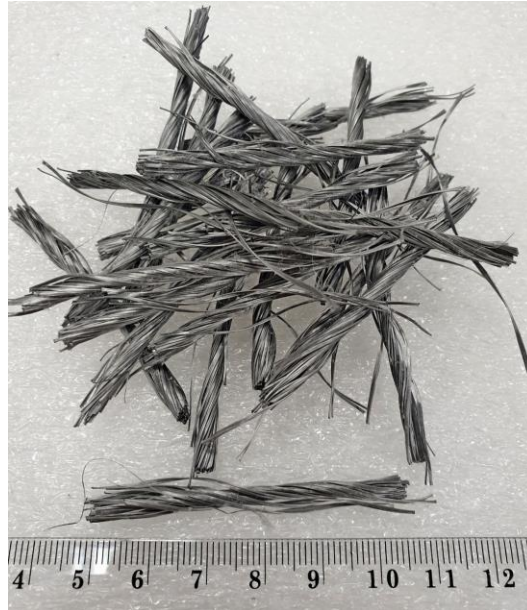
Figure 2. Photograph of twisted-bundle macro-polyolefin fibres
