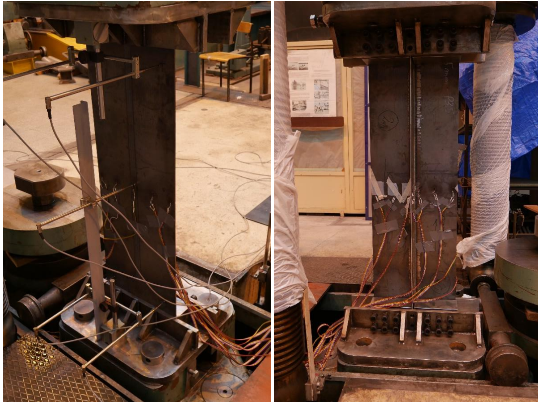
Figure 5. Back (left) and front (right) view of specimen with installed gauges.
