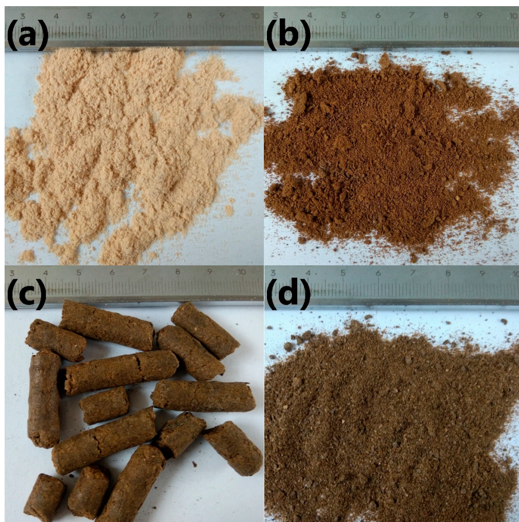
Figure 1. The appearance of the (a) beech wood flour, (b) modified brewers' spent grain, as well as coffee silverskin (c) before and (d) after grinding.
