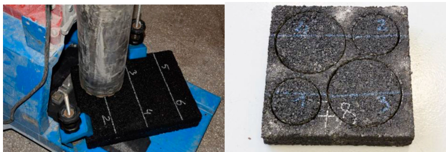
Figure 7. Coring of cylindrical specimens with a laboratory drill and an exemplary plate with cored 100 and 150 mm specimens.
