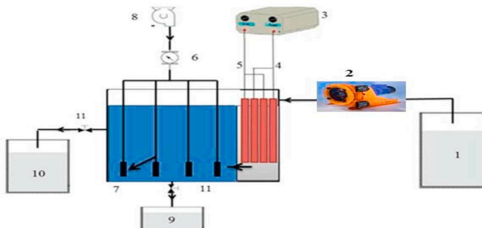
Fig. 1. Schematic diagram of the electro-Fenton-sequencing batch reactor.
