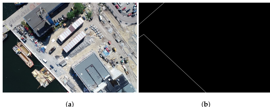
Figure 5. Coastline image: (a) on the photo with geometric distortions removed, (b) obtained as a result of perspective projection of the edge of the land area from the ENC (equivalent).
