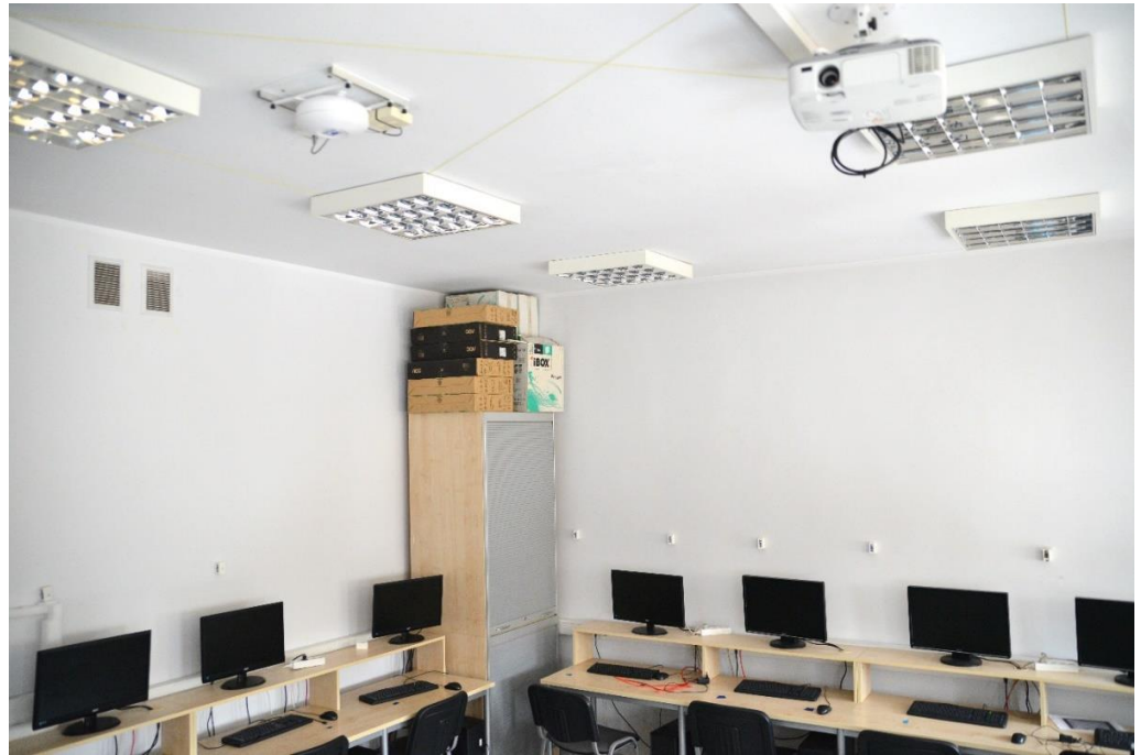
Figure 7. Test environment with reference nodes installed on the walls and the ESPAR antenna integrated with the custom-made WSN board in a single housing mounted on the ceiling.
