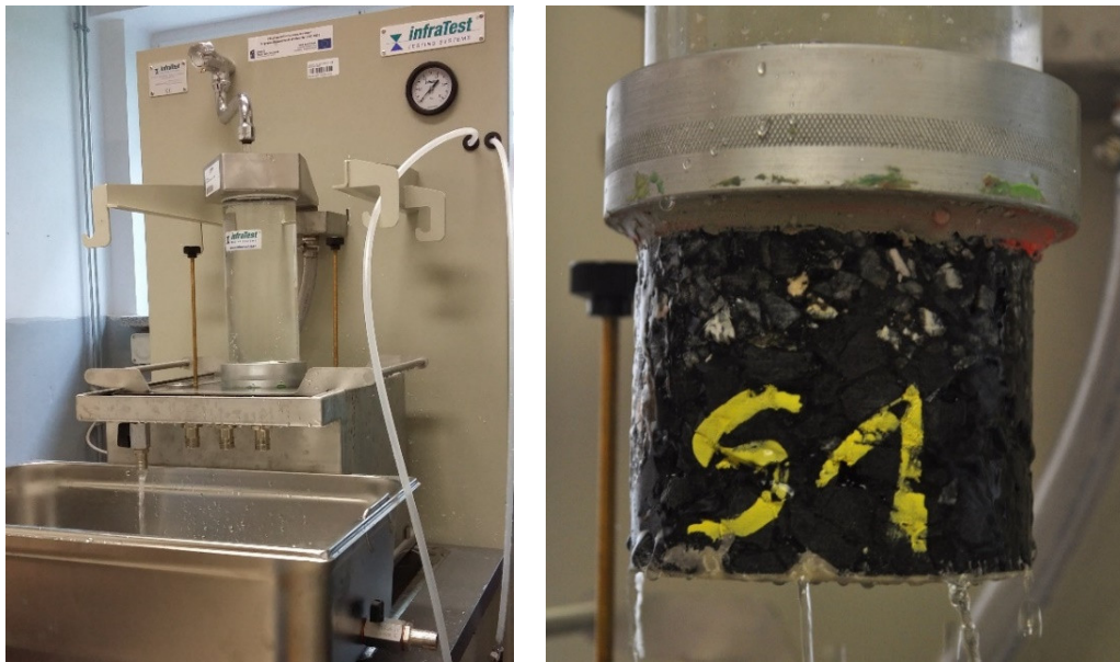
Figure 6. Vertical water permeability test.
