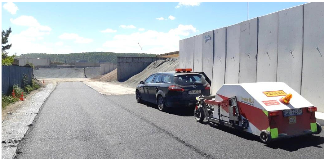
Figure 7. Tyre/road noise measurements using the CPX method.
