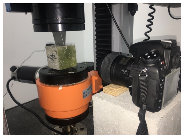
Figure 9. Test stand for testing tensile cracking characteristics when splitting concrete sample with a wedge (WSP) using digital image correlation (DIC) method.
