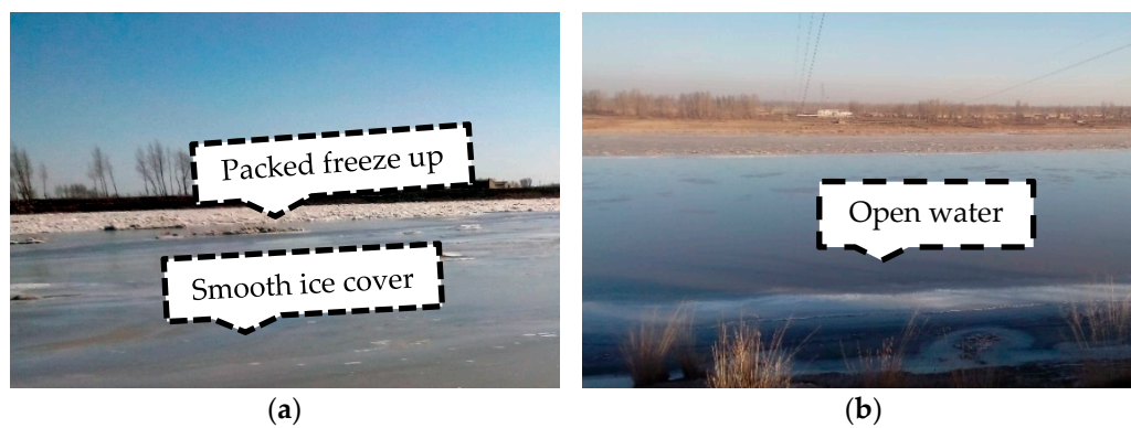
Figure 4. The freeze-up form of the Shensifenzi bend, monitored in the field. (a) Freeze-up forms in the bend. (b) Open water leads downstream of bend.
