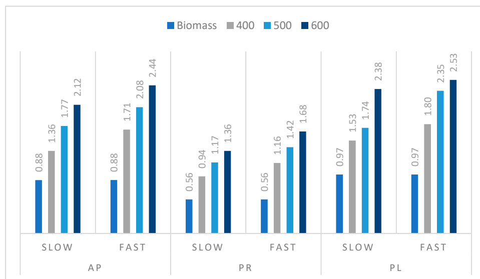
Figure 9. Raw material and biochar ash content per 1 MJ of energy ratio (g/MJ).
