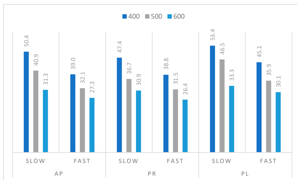
Figure 4. Biochar yield (wt %) from pyrolysis of residual biomass from tree prunings from orchards carried out at different temperatures and heating rates (slow pyrolysis—15 °C/min and fast pyrolysis—100 °C/min).
