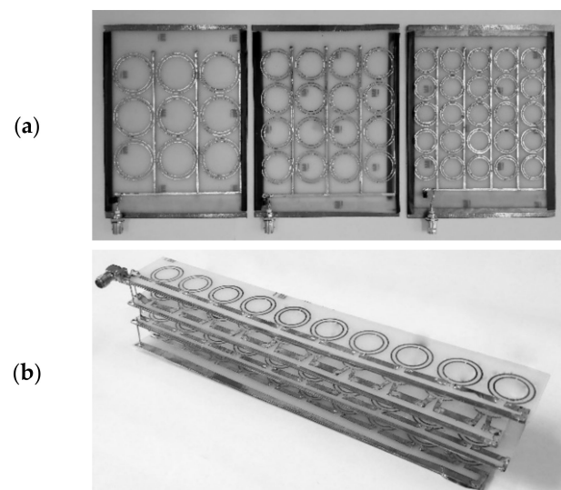
Figure 13. View of the prototypes of the (a) three frequency variants of a flat metamaterial matrix, and (b) transverse metamaterial matrix.
