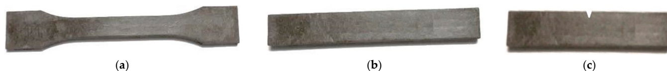
Figure 1. Samples for: (a) tensile; (b) bending; (c) impact test.
