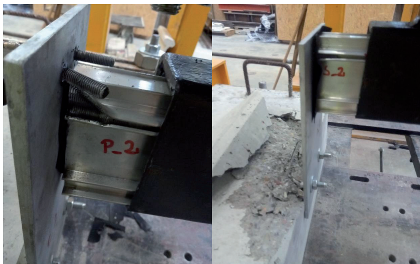
Fig. 4. Form of bracket failure: a) left – pressure, b) right – suction
