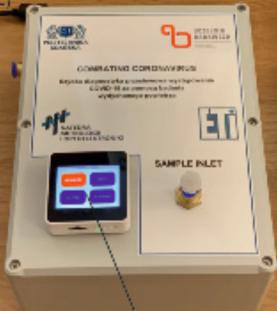
Embedded control unit M5Stack Core2 ESP32 IoT
