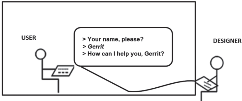
Figure 9.7. The idea of the “Wizard of Oz” prototyping (adapted from Sharp et al. 2019, Dix et al., 2004)
