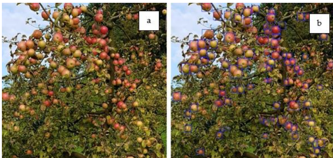
Figure 7. Example of YOLO (You Only Look Once) operation on the selected tree (a—original image, b—counted apples). Source: own study.
