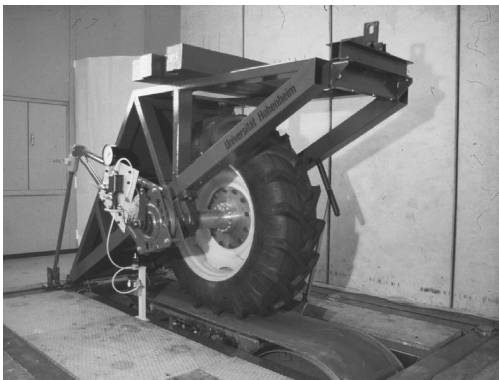
Figure 2.3 The flat belt test stand at Hohenheim University of Technology [22]
