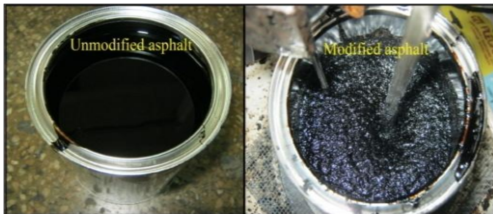
Fig. 5.5: Morphological differences between virgin and modified asphalt
