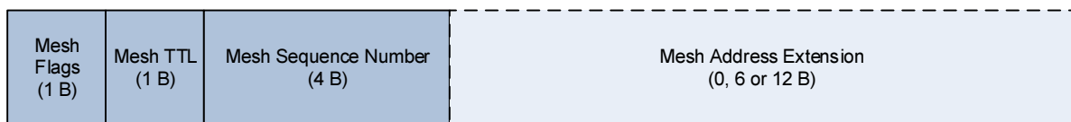
Fig. 57 Mesh Control field structure
