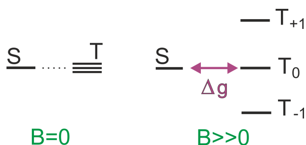
Figure 4.17. Schematic representation of the conversion mechanism of ^1(e-h) \leftrightarrow ^3(e-h) pairs in the case of the \Delta g mechanism
