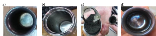
Fig. 4. Calorimetric bomb crucibles with residues of combustion products: a) MDO (Gdańsk University of Technology laboratory), b) RMD 80/S (Gdańsk University of Technology laboratory), c) RMG 380 (Gdańsk University of Technology laboratory), d) RMG 380 (LOTOS laboratory)
