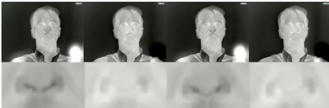
Figure 6.4. Every \sim 45^{th} frame (inhalation/exhalation event can be observed every \sim 3 seconds, FPS=15) extracted from SC3000-ADRA-8-test sequence magnified with EVM; inhaled air is colder, thus nostrils have darker color; exhaled air is warmer (heated by body), thus nostrils are lighter
