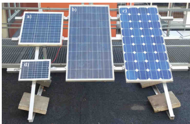
Fig. 2. Photovoltaic modules in natural dust study: a - MWG-30, b - AP-7105, c - STP-085, d - CLC010-12P
