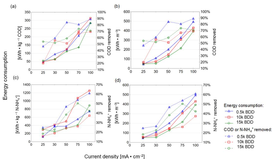
**Figure 9.** Energy consumption after 8 h of EO process using different BDD/Si electrodes and different current densities plotted against COD removed (a,b) and N-NH<sub>4</sub><sup>+</sup> removed (c,d).
