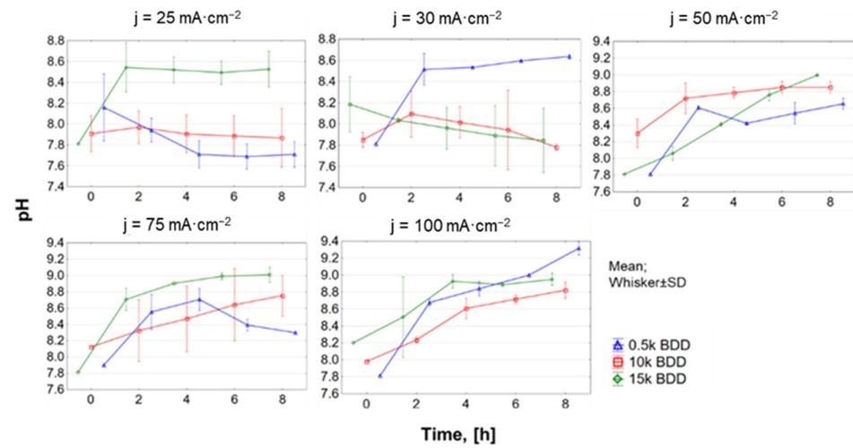
Figure A4. pH changes in LLs with different BDD anodes and current densities (25–100 mA·cm<sup>-2</sup>).
