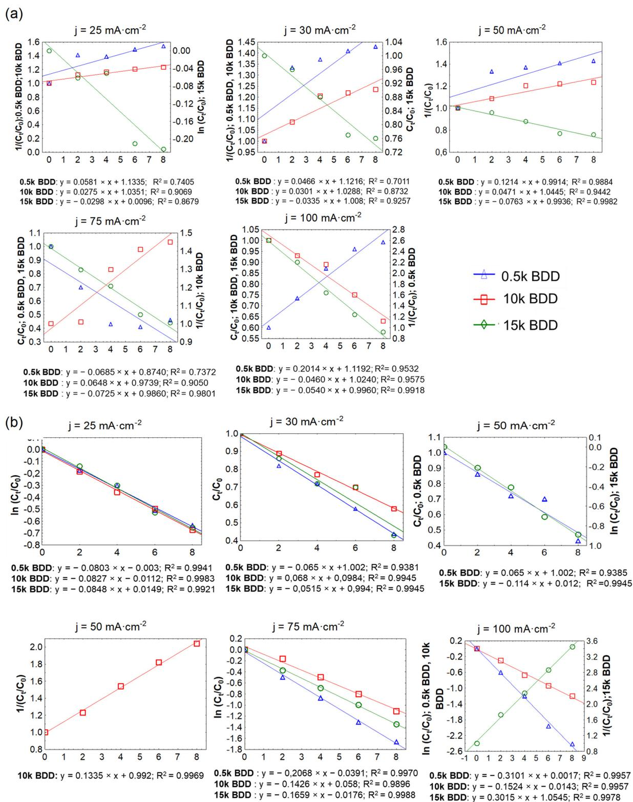
Figure 8. Determination of the order of removal of: (a) COD and (b) N-NH<sub>4</sub><sup>+</sup> by the graphical method.
