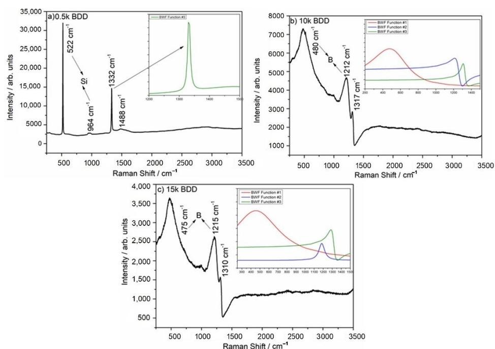
**Figure 3.** Raman spectra of (a) 0.5 k, (b) 10 k, and (c) 15 k BDD films. Insets shows Raman spectra modeled using Breit–Wigner–Fano function: Fano-shaped peaks (BWF #1 red line, BWF #2 blue line, and BWF #3 olive line).
