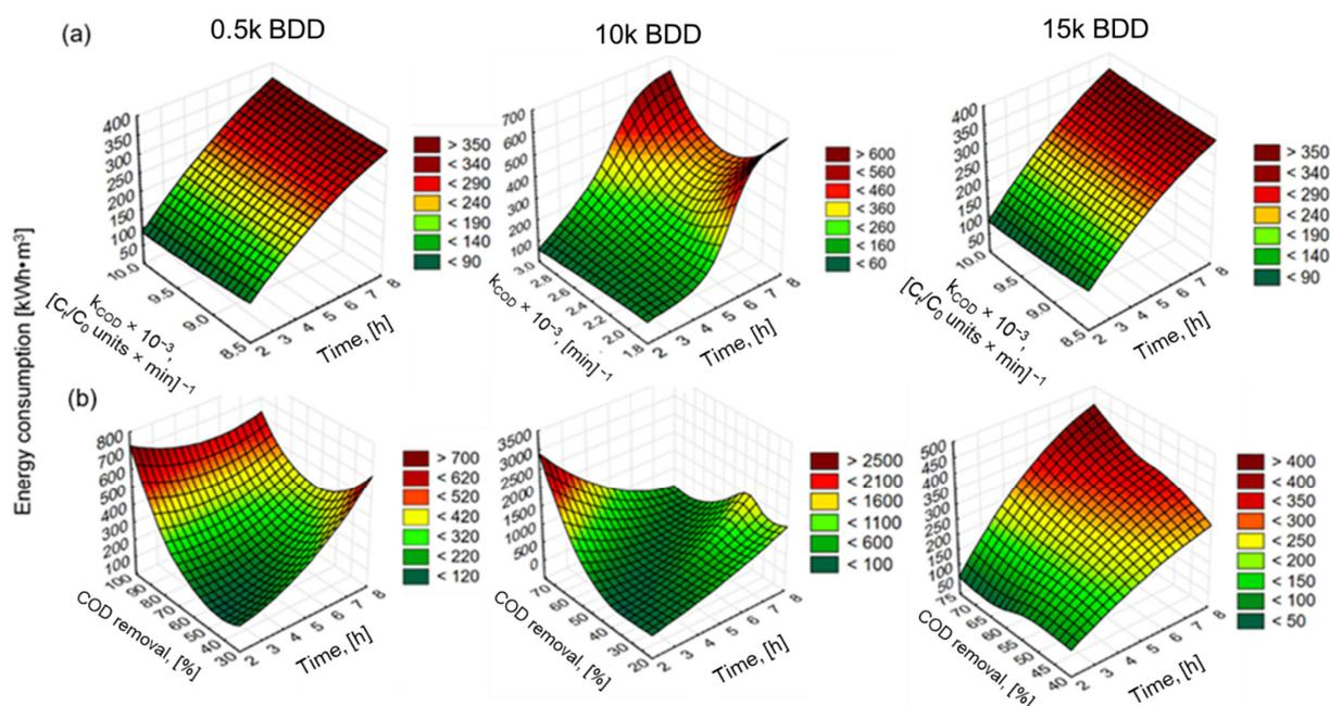
**Figure 10.** Surface plots (distance weighted least squares) of: (a) energy consumption against constant rate coefficient and time of EO and (b) energy consumption against COD removal efficacy and time of EO for  $j = 100 \text{ mA}\cdot\text{cm}^{-2}$  and different electrodes used.
