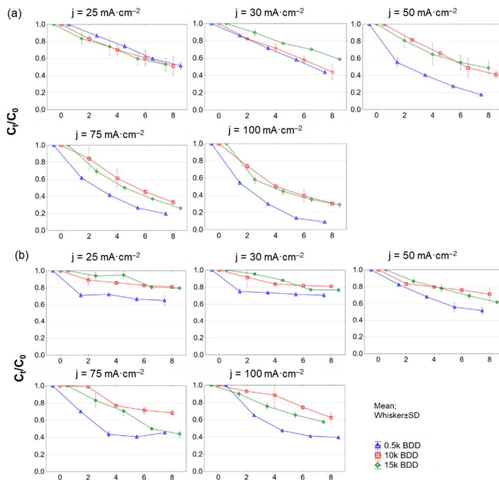
**Figure 5.** Removal of (a) COD and (b)  $N-NH_4^+$  during 8 h test of LL treatment with different BDD anodes and current densities ( $25\text{--}100\text{ mA}\cdot\text{cm}^{-2}$ ) expressed as normalized concentration  $C_t/C_0$ .
