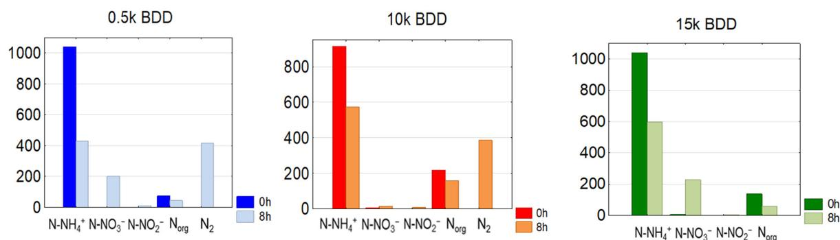
**Figure 7.** Average  $C_0$  and  $C_{8h}$  concentrations of nitrogen compounds in treated LLs by means of different anodes used,  $j = 100 \text{ mA}\cdot\text{cm}^{-2}$  ( $N_{\text{org}} = \text{TN} - (\text{N-NH}_4^+ + \text{N-NO}_3^- + \text{NO}_2^-)$ ).
