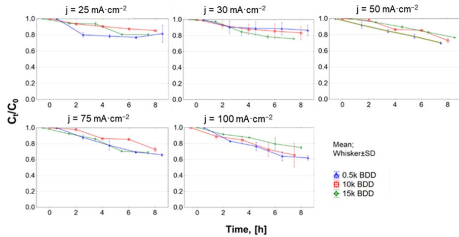
Figure A3. TN changes in LLs with different BDD anodes and current densities (25–100 mA·cm<sup>-2</sup>).
