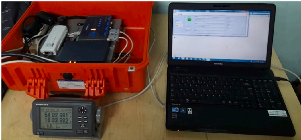
Fig. 9. Real-time satellite navigation data recording system.
