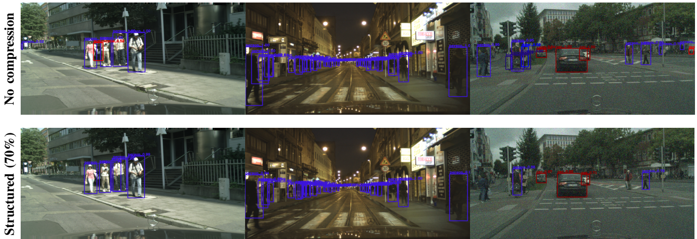
Fig. 5: Detection samples for base model and the model structurally pruned at 70% compression rate. Detections on the original Cityscapes dataset (first column), ECP dataset (second column) and noise distortion (third column).
