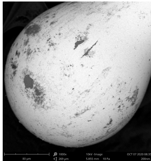
Figure 1. SEM image of the microsphere sensor with a 100 nm ZnO ALD coating. Magnification of 1000 \times .
