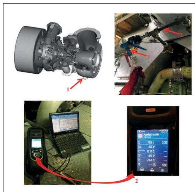
Fig. 10. Method of introducing the measuring probe of the exhaust analyser into the turbine exhaust duct of the turbocharger in the tested engine (a) and the view of the measurement set during the test realisation (b): 1 - drainage channel [21], 2 - magnification
