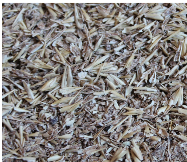
Fig. 6 The appearance of BSG without additional treatment
