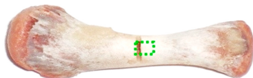
Figure 2. Extracted chicken humerus prepared for the reference OCT measurement. The green rectangle indicates the scanned region.
