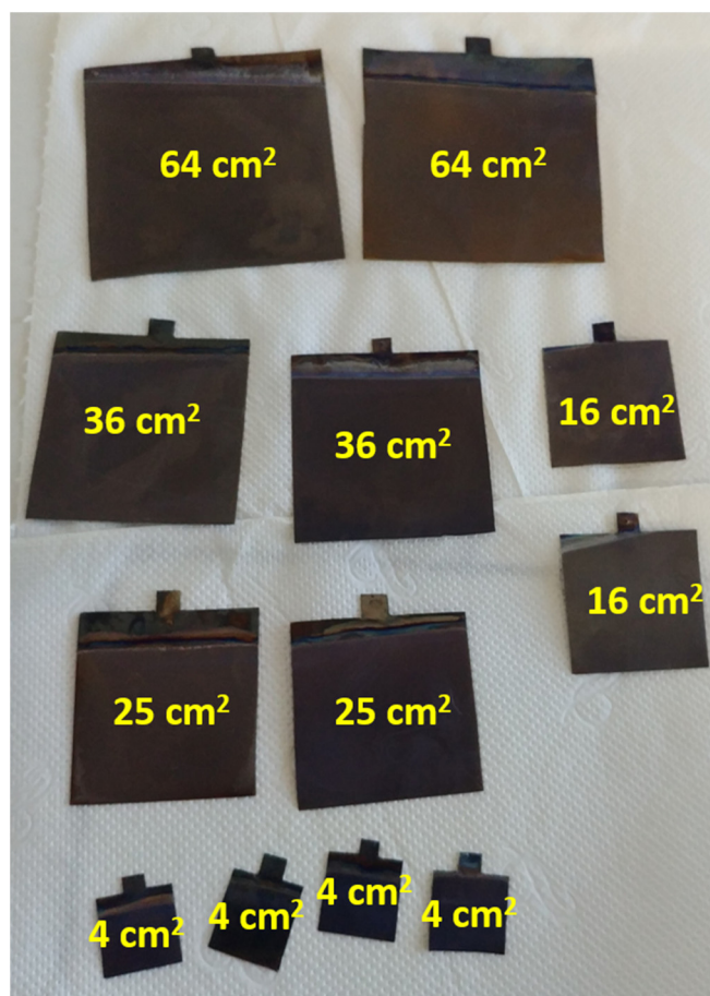
Figure 1. Titanium foil (of different dimensions) after the anodization and calcination process.
