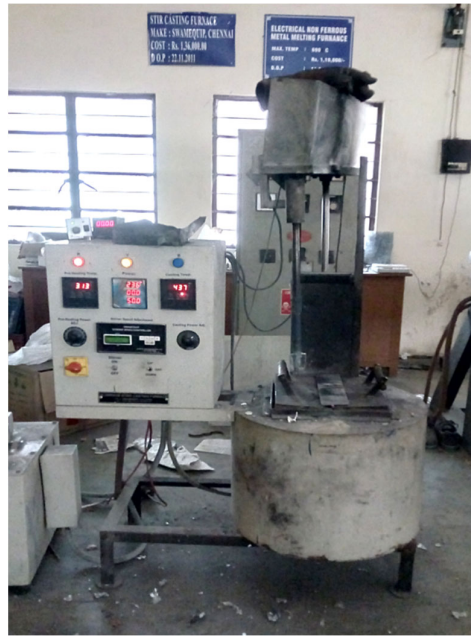
Figure 1. Stir casting setup.
