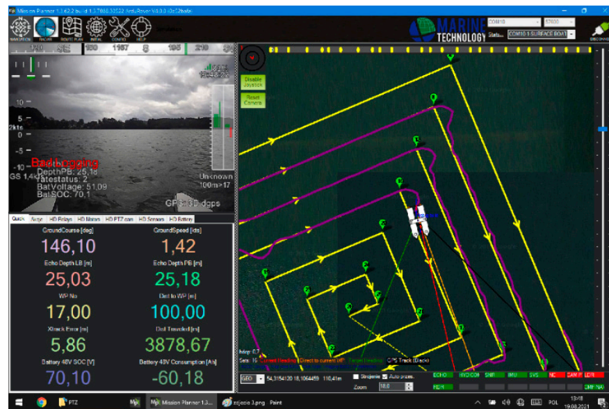
Figure 6. Window of the ArduPilot Mission Planner application used for the planning and recording of a vessel's route.
