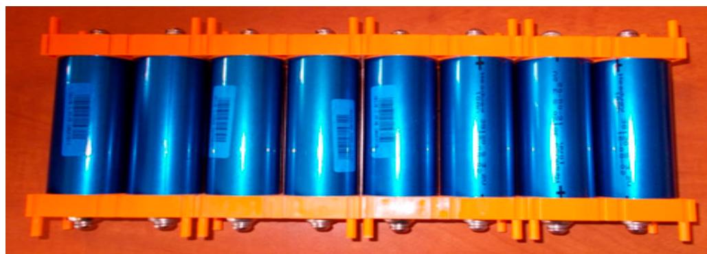
Figure 5. Battery pack arranged of eight lithium-iron-phosphorous (LiFePO 4 ) cells for testing.
