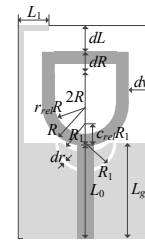
Fig. 22. Geometry of the ultra-wideband antenna [65]. Ground plane marked using light gray shade.
