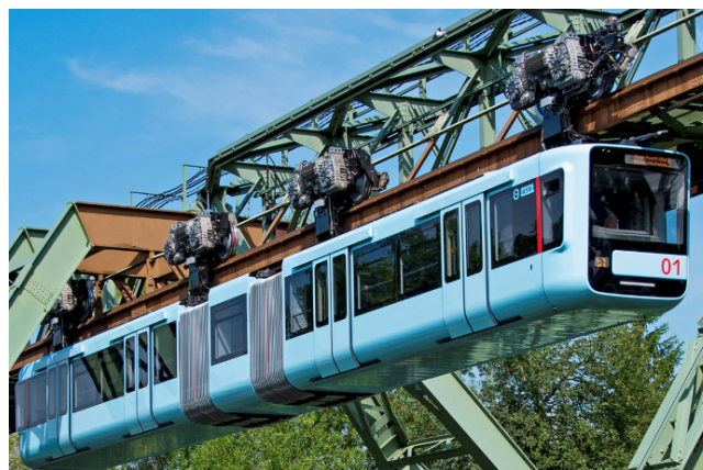
Fig. 1. Vehicle of Eugen Langen system – G 15 [2] Rys. 1. Pojazd systemu Eugen Langen – G 15 [2]
